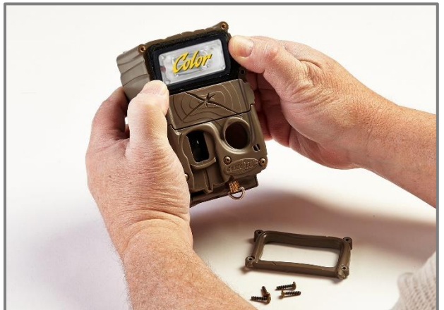
STEP 4: Gently push the new flash module in to make secure
