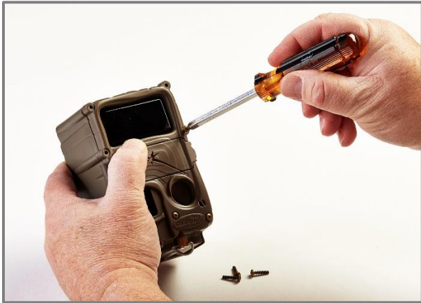
STEP 1: Unscrew the 4 x screws on the flash cover
