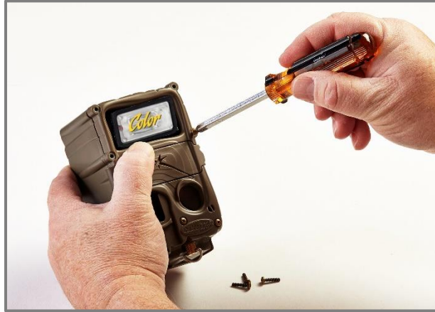
STEP 5: Tighten the 4 x screws on the flash cover
