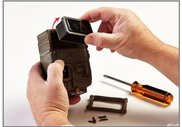
STEP 2: Gently pull out the existing flash module
