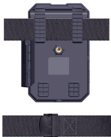
Figure 8: Mounting the Camera
