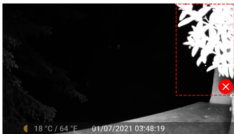
Figure 7: Avoid close-up obstacles in front of the camera
